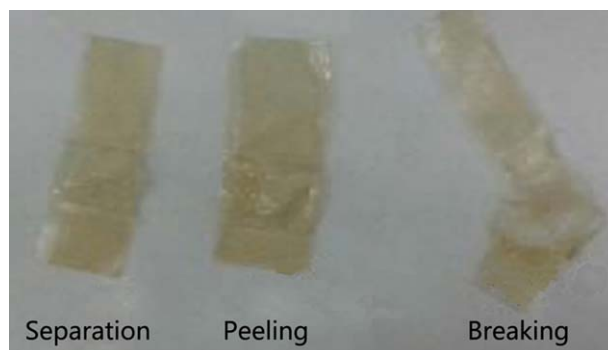
Figure 4. Three failure modes observed, from left to right, are separation, mode A (peeling), and mode D (breaking). [Color figure can be viewed in the online issue, which is available at wileyonlinelibrary.com.]
